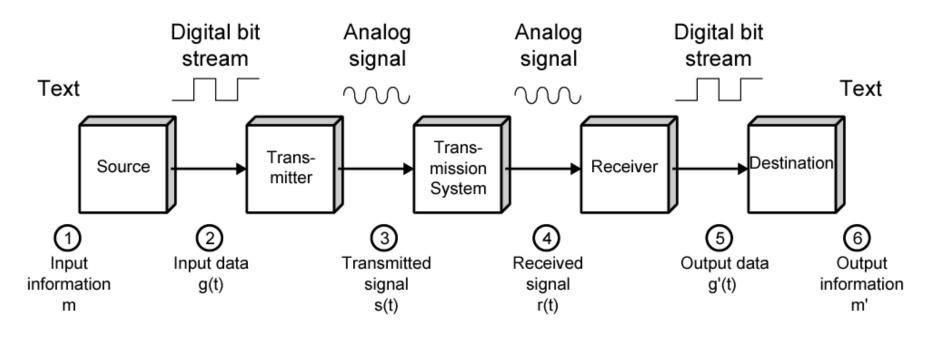
A distortion-less communication system is one for which m' is an exact replica of m. The task of the system is to minimize the difference between m and m' in the presence of noise, i.e., to minimize the distortion :  $E(m - m')^2$ ; MSE
